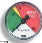
MC-20 RETURN LINE INDICATING GAUGE FOR 25 PSI FILTER APPLICATIONS 2" MULTICOLOR 0-20 PSI GREEN 21-24 PSI YELLOW 25-60 PSI RED (SERVICE FILTER)
